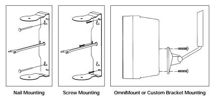
Figure 7 The OS3 can be mounted three ways.
